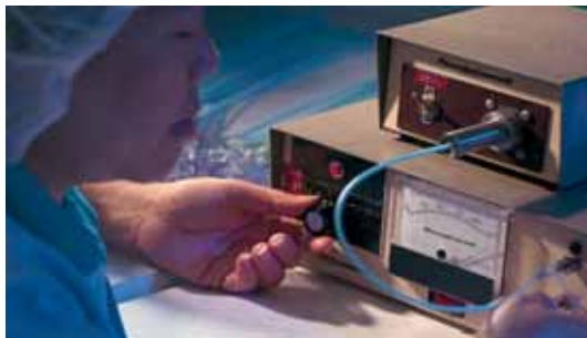
Every Life-Tech urodynamic catheter is hand tested for lumen integrity, crosstalk and patency.
