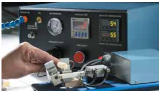
Automated control of heat, pressure and application time ensures uniform, high strength bonds.
